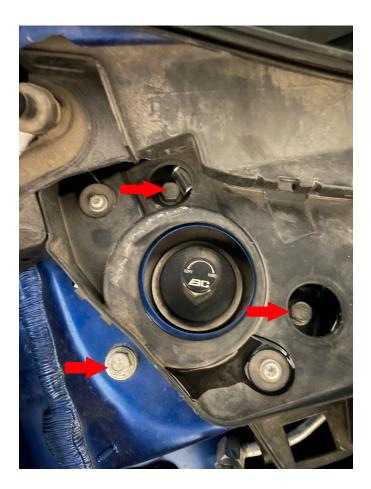
When these bolts are removed the shock will fall freely, be sure to support the bottom of the shock by either using the jack or by holding the shock body when removing the last bolt.
