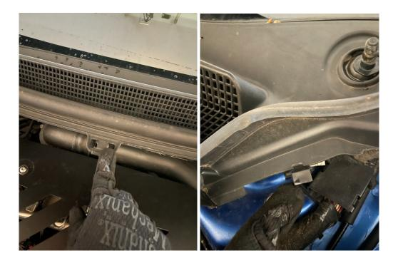
The 3 13mm bolts for the top mount should now be easily accessible. Removing these bolts will come in a later step.
