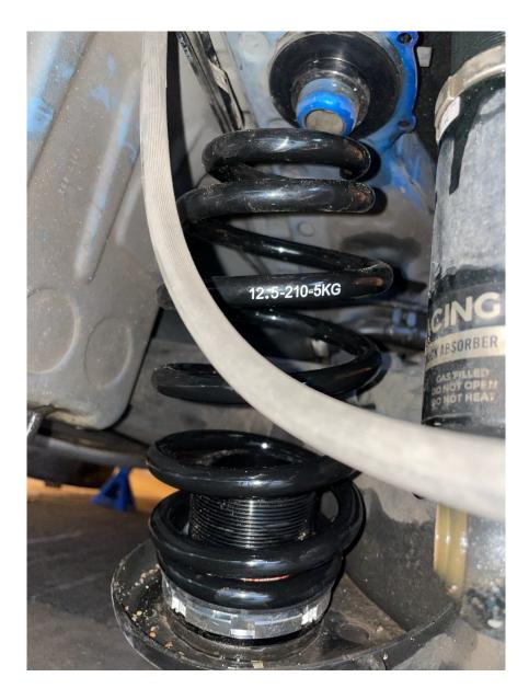
5.) Place jack under the rear spring seat and slowly raise the rear axle. While raising the axle make sure the top of the springs seat properly. Raise the axle until the spring is compressed approximately 5mm.
