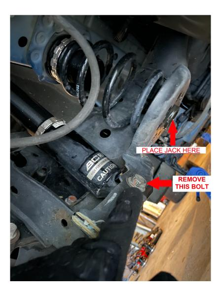
2.) Once 18mm bolts are removed, slowly lower the jack. The axle should fall freely uncompressing the springs. Once the springs are fully uncompressed and the axle is free hanging remove the springs.
