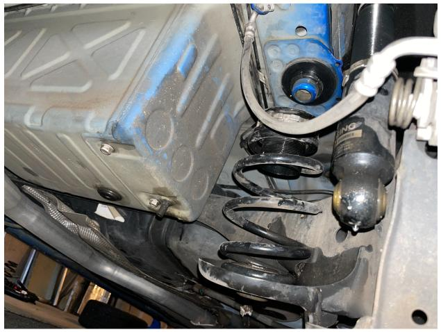
Do not discard these rubber bushings from spring seats as you will be reusing them with the new springs. There is a bushing on both the top and bottom spring seats.
