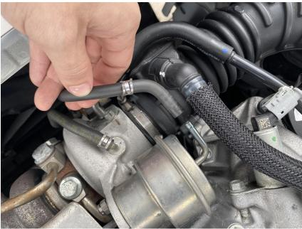
3. Remove the 2 10mm bolts holding the stock actuator in place, and also remove the retainer clip on the wastegate arm, which you should be able to work out by hand. Do not lose this retainer/pin as you will reuse it.
