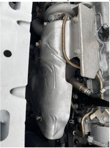
2. Remove the boost/vacuum line attached to the stock actuator by using pliers to release the clip and sliding it off of the actuator, allowing you to pull the line off of the fitting, it is recommended that you leave the clip a good distance back on the hose to make install of the BNR actuator easier.
