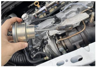
4. Determine which of the two supplied turnbuckles fit your wastegate flap arm, note that the fit should be snug with no play between the two pieces.
