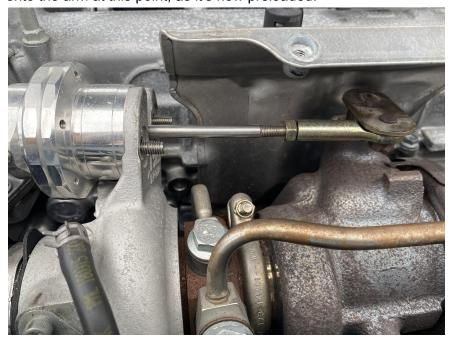
7. After you've got the actuator fitted to the wastegate arm and you're happy with the tension just simply put everything back together, make sure to move the metal clamp back over the actuator with the rubber intake hose. If you have a BNR tune, you should be seeing 21-23psi of boost at wide open throttle. Tighten or loosen the arm as needed to make the desired boost.
