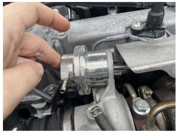
DO NOT reinstall the hose or tighten the actuator down at this point.
