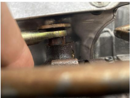
5. Once you've determined which turnbuckle to use, thread it onto the actuator followed by the fitting, you can ascertain an approximate thread depth by holding the actuator up to the turbo as shown in the picture. Once you have it close you can put the actuator into place making sure that the intake port on the top is facing outward.
