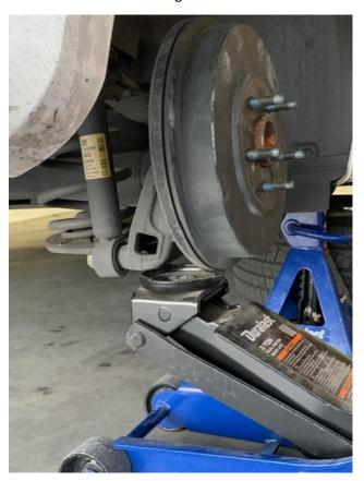
3. Place jack under rear hub assembly as shown in picture. Raise jack until it makes firm contact with assembly. This will allow you to remove the shock without the assembly falling.
