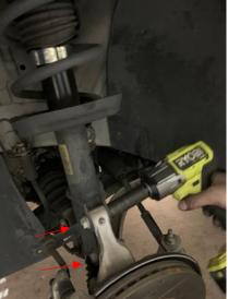
9. The bottom of your strut is held on by 2 19mm bolts and 2 19mm nuts. Use your socket and wrench to remove these bolts. When removing bolts, be sure to keep control of your strut assembly as it will fall freely from vehicle.
