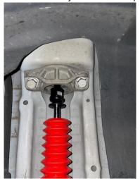
5. For upper shock removal, there are 2 18mm bolts that need to be removed. You may have to bend your fender liner back to reach the aft bolt properly.
