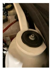
6. Once under hood, you will see the upper strut mount. This is held in place by a 24mm nut. Remove the nut with 24mm socket. If assembly turns freely, it may be necessary to hold strut in place with T40 while turning 24mm nut with wrench. Once removed, your jack will now support the weight of the hub assembly.
