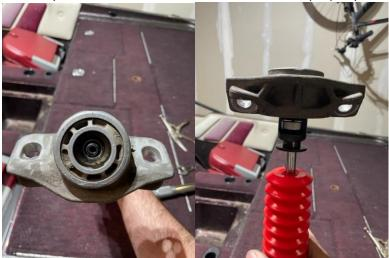
6. Once removed, you will want to remove the upper mounting bracket from the old shock so it can be reused. At the top of the shock is a 15mm nut. Remove this nut and the bracket will come off. If the nut spins the shock, use a pair of vice grips to hold shock in place while loosening nut. Install bracket to new shock with supplied 17mm nut.
