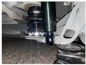
4. Using a 21mm socket, remove lower shock bolt. It will decompress slightly when the bolt is removed. Your jack is now the primary support for the assembly's weight.
